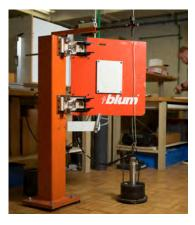
Wear and Fatigue testing aren't the only tests our hinges are subjected to in our lab. Weighted tests ensure hinges hold up to the treatment life will inevitably put them through. Have you ever noticed yourself using a cabinet door to help hoist yourself back up after squatting down to look for an item? We've all done it, and often without thinking about it. Blum actually mimics these situations during testing.
