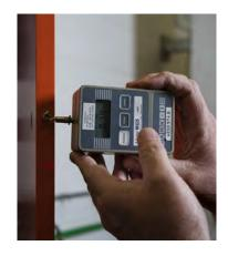
For both hinges and drawer runners, we measure the opening and close forces needed for optimum function of Blum products. Digital gauges track the amount of force needed to open and close a door or drawer. By doing so, we ensure the cabinet remains closed, can be easily pulled open and closes as softly as designed.
